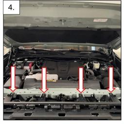
5. Remove the electrical connectors from the top of the grill near the top of the radiator. For TRD models, there are two on the driver side and two on the passenger side. For non-TRD models, there are two on the passenger side and one on the driver side.
