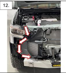
13. Run the switch lead along the firewall and to the wiring passthrough located to the right of the brake master cylinder.
